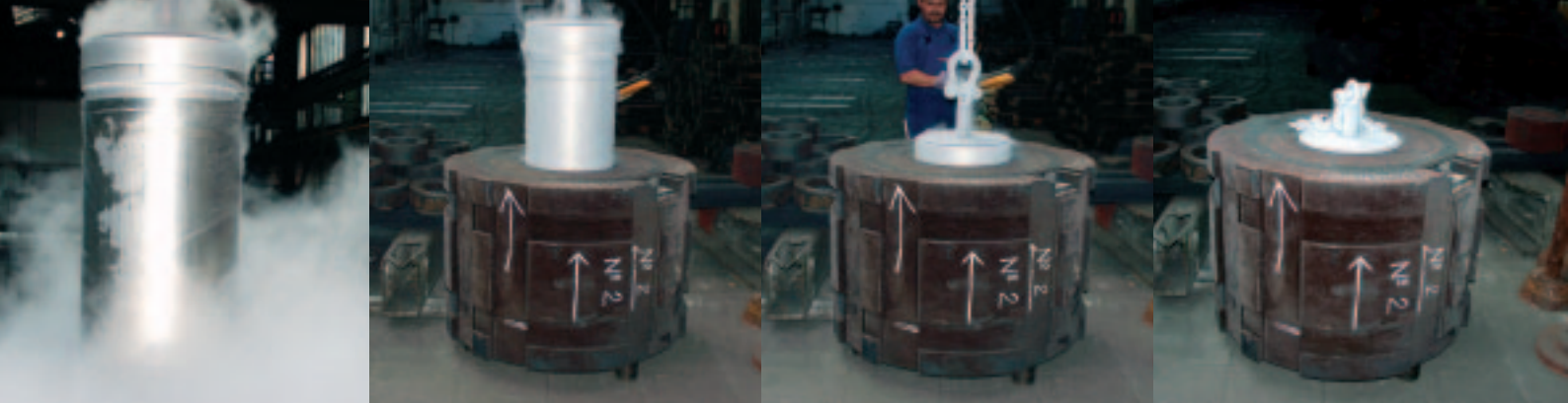
Supercooled shrinking of inner liner with double shoulders
