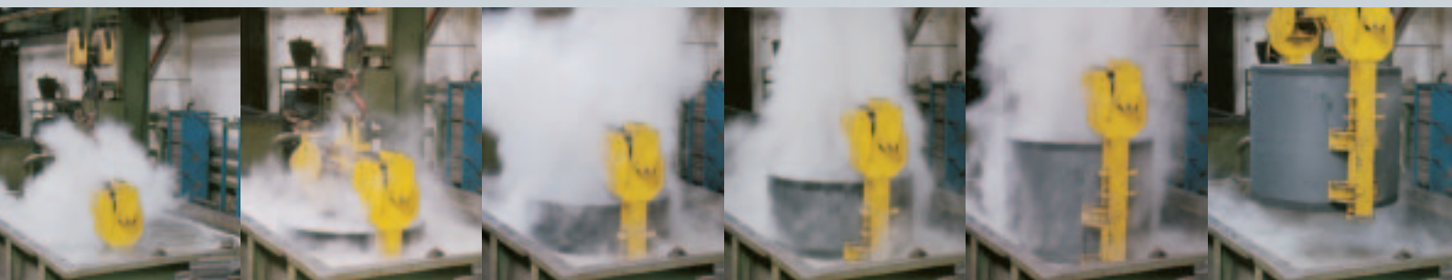
Quenching of a mantle in a polymer bath
