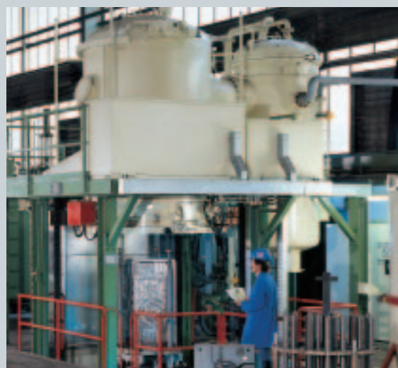
Vertical loading for low-distortion vacuum hardening
