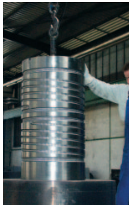
Shrinking of a cooled intermediate bushing in a preheated jacket
